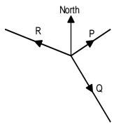
**P** is of magnitude 350N on a bearing of 060°, **Q** is of magnitude 600N on a bearing of  $\theta$ , where  $090^{\circ} < \theta < 180^{\circ}$ , and **R** is of magnitude *x* N on a bearing of 285°.
